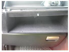
**4**. Remove the insert by pulling on the sides ensuring the clips underneath are free.
