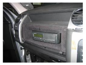
**13**. The tachograph is secured to the top or bottom of the upper glove box which is drilled for the mounting holes and cables.
