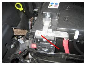
8. Bolt the +12V, A1 of the tachograph and the Red wire of the M1N1 Adaptor, through a 1 amp fuse to the spare battery terminal.
