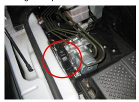
Locate the ABS pump under the left hand cover in the engine bay. Unplug then remove the AMP connector cover.
