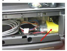
5. The M1N1 Adaptor must be secured in the gap above the upper glove box shown above.
