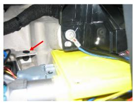
**16**. The Adaptor must be sealed to a non removable part of the vehicle by drilling a hole in the chassis shown.
