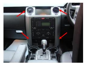
1. Remove the facia around the radio by sharply tugging on the edges indicated.
