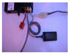
21. The cable harness is connected directly inline with the tachograph power cable when connecting to the tachograph as shown.
