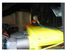
7. Ground A5 & A6 of the tachograph and the Black wire of the M1N1 Adaptor to the chassis using the bolt behind the glove box.
